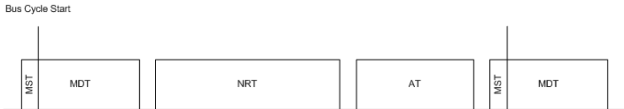
Figure 20: Diagram of MDT/NRT/AT auto-calculated Timing with maximum sized NRT Channel
